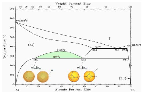
**Figure 3.** The phase diagram Al–Zn [19]. The Al(Zn) solid solution region with the *fcc* structure contains a miscibility gap with two-phase region (colored). The boundary phases with 17 and 59 at. % Zn constructions of FS–BZ are given with a common view and a view along a\* (see text).
