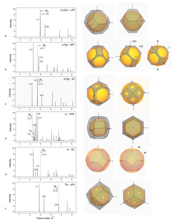
**Figure 1.** Calculated diffraction patterns for selected phases from Table 1 (left panel) and corresponding Brillouin–Jones (BZ) zones with the Fermi spheres (FS) (right panel). The position of  $2k_F$  and the hkl indices of the planes used for the BZ construction are indicated on the diffraction patterns. Constructions of BZ–FS are given in common projection (first column) and in special projection (second column) (see text).
