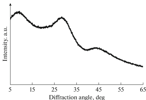
Fig. 1. XRD diffraction pattern of as-quenched CaO–SiO 2 –B 2 O 3 sealant.
