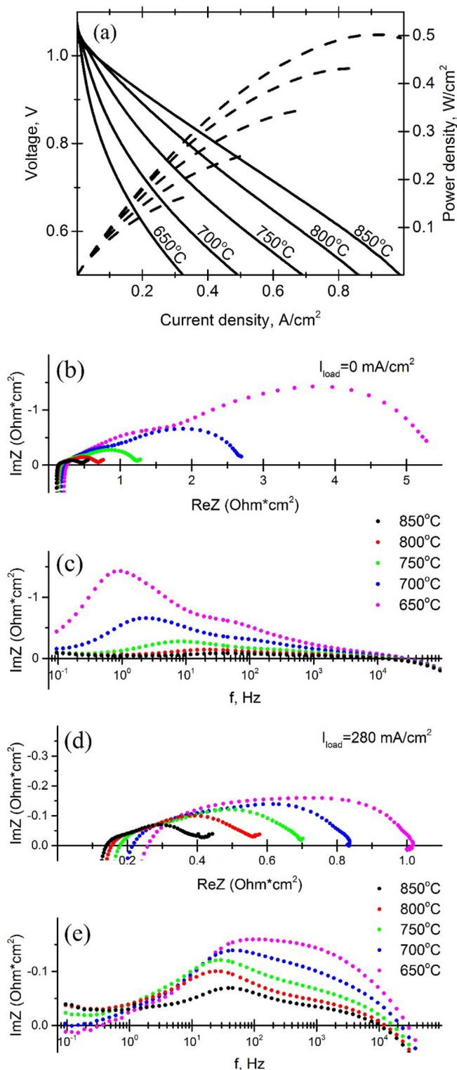
**Fig. 3.** (a) I-V and power curves of model SOFCs measured for different working temperatures from 650 to 850 °C. (b–e) Impedance spectra and ImZ over frequency dependencies for OCV conditions (b, c) and under 280 mA/cm<sup>2</sup> current load (d, e) for different temperatures.
