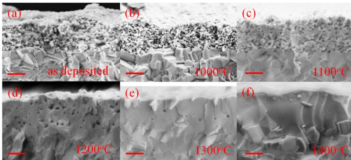
Fig. 1. SEM images of 8YSZ electrolyte film cross-section after deposition (a) and after annealing at 1000 (b), 1100 (c), 1200 (d), 1300 (e) and 1400 °C (f); the bar length corresponds to 1 μm.
