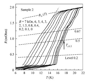
**Fig. 1.** The R(T) curves for sample 2 in magnetic fields (from right to left) from 0 to 7 kOe. The dashed lines are the straight line  $R_n(T)$  and the straight lines at the levels of 0.67, 0.5, and 0.2 of  $R_n(T)$ . The method of determining the onset of the transition is demonstrated, and the  $T_{ci}$  fields from which the shifts were measured are shown.
